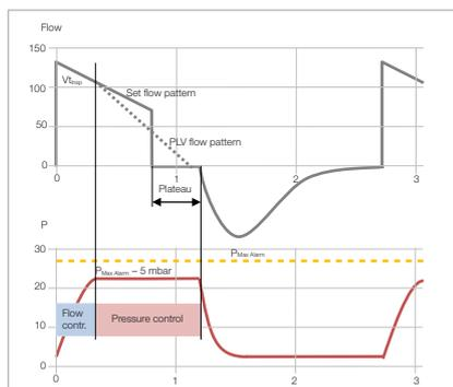
PLV is automatically enabled with volume-controlled breaths. As soon as the inspiratory pressure rises to 5 mbar below the set  $P_{Peak}$  alarm, the pressure is kept at that level until the set tidal volume has been reached, but until the end of the set inspiratory time at the latest. Plateau time is shortened as far as necessary. A blue info message is displayed when enabled with PLV. If the set tidal volume cannot be reached, an appropriate alarm message appears.
