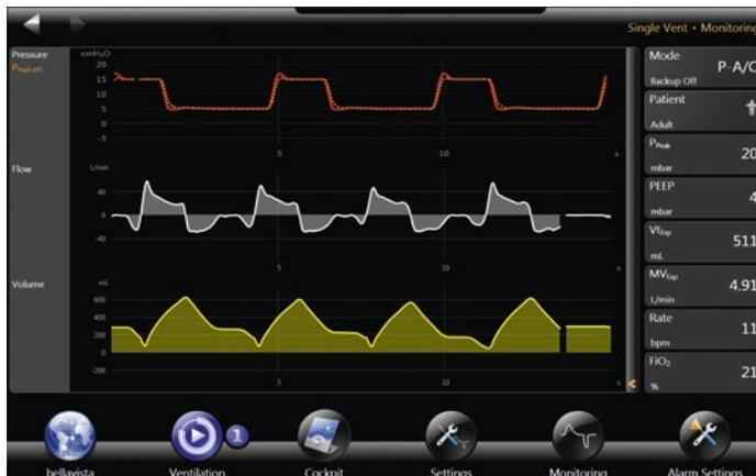
The calculated  $P_{ATC}$  curve is superimposed on the pressure curve
