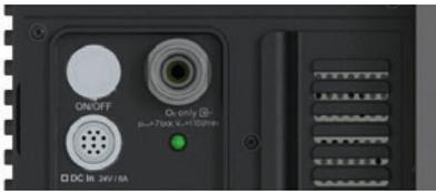
Switch on bellavista with the “ON/OFF” button on the left-hand side of the device. Start-up takes ≈1 min.
