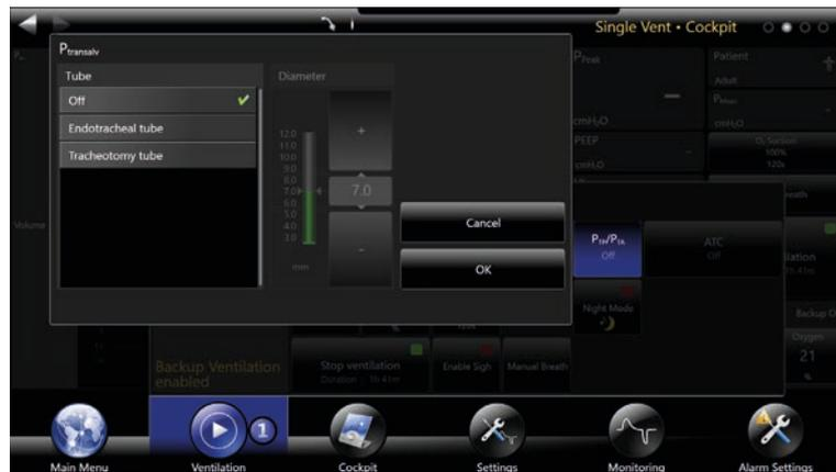
Activation and setting tube diameter with the  $P_{TP}/P_{TA}$  button
