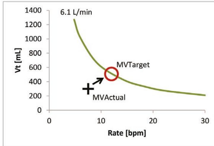
Lung protective safety range for target rate and target tidal volume
