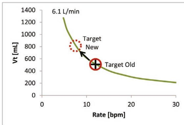
After a change in the patient's respiratory mechanics, AVM adapts rate and tidal volume while maintaining the target minute volume
