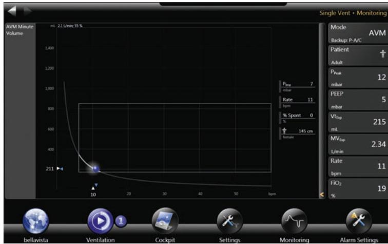
Monitoring screen configured for AVM. The white arrows indicate target rate and tidal volume whereas blue indicates actual rate and tidal volume.
