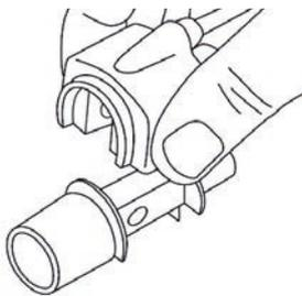
Attach the CO<sub>2</sub> respiratory gas sensor to the airway adapter
