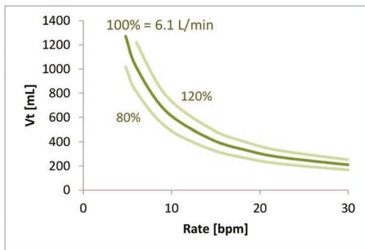
Target minute ventilation curve for 80% MinVol, 100% MinVol and 120% MinVol at an exemplary nominal minute volume of 6.1 L/min
