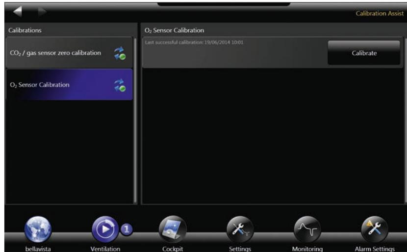
**Warning:** An incorrectly calibrated CO<sub>2</sub> sensor may lead to incorrect CO<sub>2</sub> respiratory gas measurement.
