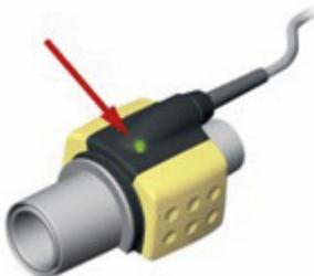
The green LED indicates that the device is ready for operation
