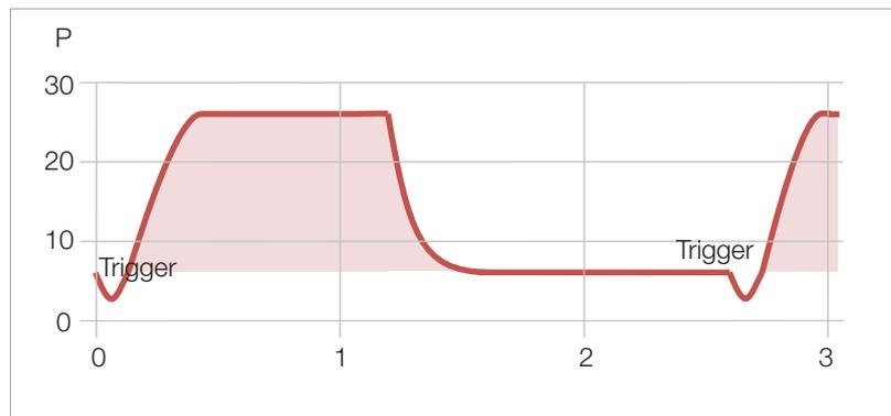
With synchronised breaths the curve is displayed as a filled curve
