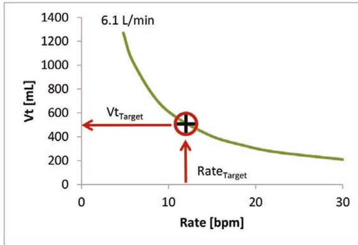
Calculation of optimal target rate (Otis' equation) and subsequently target tidal volume for an exemplary minute volume of 6.1 L/min
