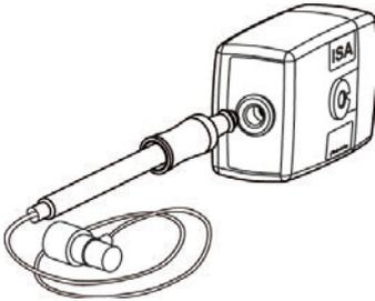
Connect the Nomoline measuring line to the ISA input
