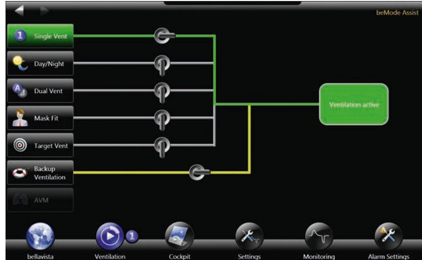
beMode Assist: higher-level behaviour of various device functions and options.
