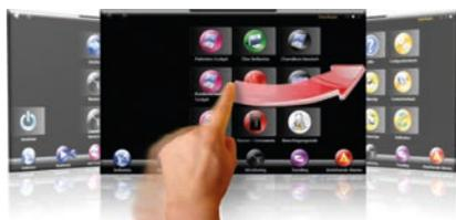
With a horizontal swiping motion across the touch screen you can scroll from screen to screen.
