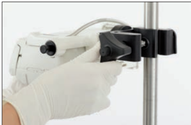
Attaching Pole Clamp to IV Pole Position the opening of the Pole Clamp on pole and turn black knob clockwise until pole clamp is secured to IV pole. Turn black knob counter clockwise to release from IV pole.
