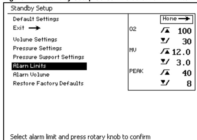
2. Select and confirm the desired alarm limit (Figure 122).
