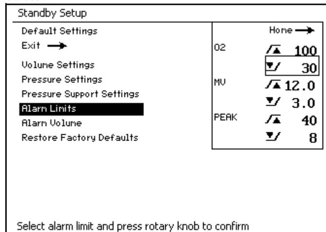
3. Select a new setting value (ex., in Figure 123, the setting value was changed from 30 to 25).
