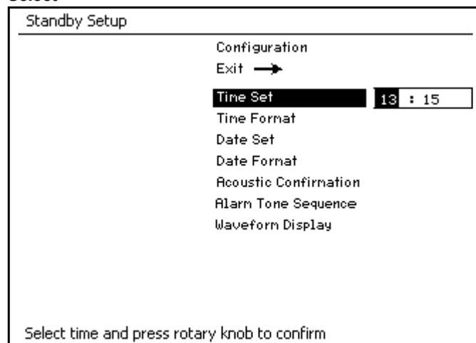
Figure 129. Standby Setup Screen Configure Time Hour
