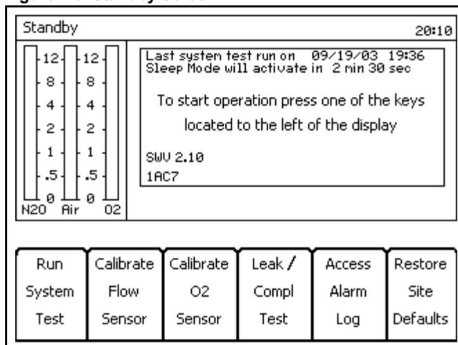
Figure 14. Standby Setup Screen
