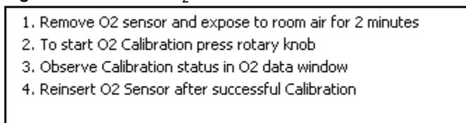
Figure 93. Calibrate O<sub>2</sub> Sensor in Progress Bar
