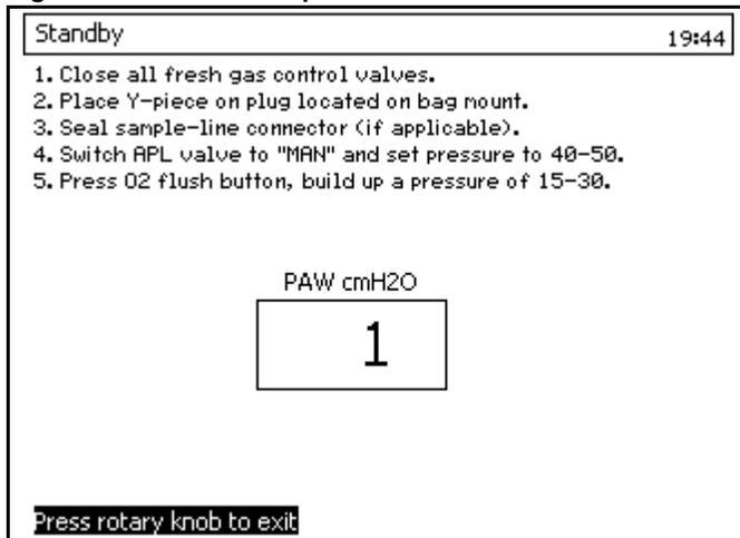
Figure 113. Leak / Compliance Test Results Screen
