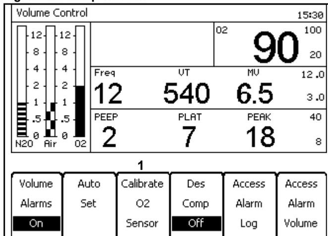
Figure 81. Calibrate O<sub>2</sub> Sensor Instruction Screen
