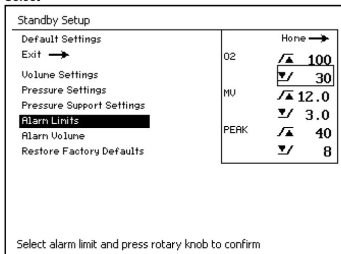
5. Confirm the alarm limit value and select a new value for the alarm limit (ex., in Figure 18, the value was changed from 30 to 25).
