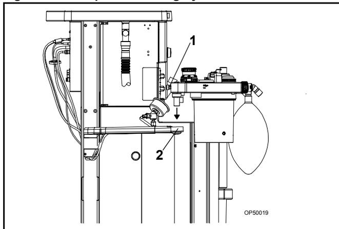
Figure 52. Hose Connections for Compact Breathing System
