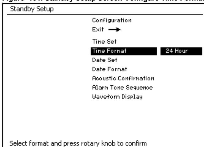
2. Select and confirm a new time format value (ex., in [Figure 129](#), the value is changed from “24:00 Hour” to “AM/PM”).
