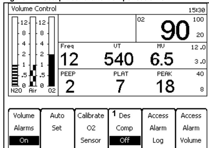
Figure 95. Setup Desflurane Compensation On
