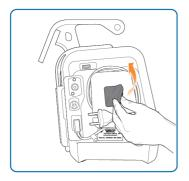
Figure 12-3. Step 3. Remove back panel.
