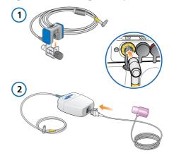
Figure 5-9. Sensor and adapter connected for calibration
