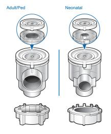
To assemble/install the expiratory valve
