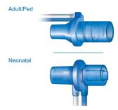
The area of the orifice changes depending on the flow rate. It opens progressively as the flow increases, creating a pressure drop across the orifice. The pressure difference is measured by a high-precision differential pressure sensor inside the ventilator. The pressure difference varies with flow (relationship determined during flow sensor calibration), so the patient's flow is determined from the pressure drop. The ventilator calculates volume from the flow measurements.
