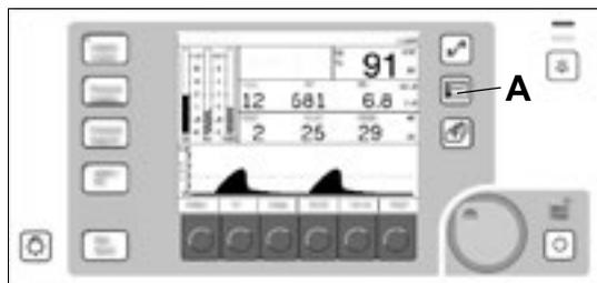
The volume alarms can be switched on and off during operation by pressing the
