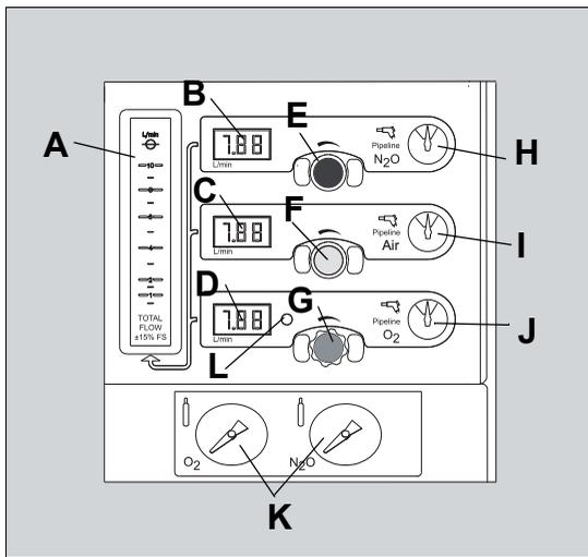
**K** Pressure gauges for gas cylinders (only for devices on trolley)\*
