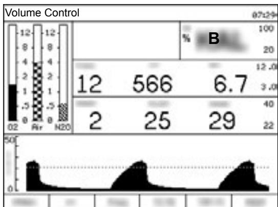
During the calibration, the O2 value in the window (B) of the O2 monitoring is replaced by the word **CAL**. The calibration time is approx. 15 seconds. After successful calibration, the O2 measured value is again displayed.
