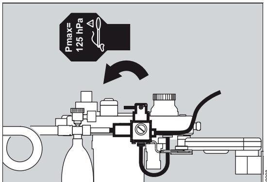
Diverting the fresh-gas flow to the non-rebreathing system:
