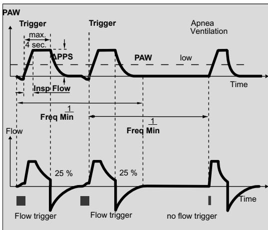
If the inspiratory flow (**Insp Flow**) during inspiratory effort is greater than the set trigger flow (**Trigger**), the device supports the patient with the setting  $\Delta PPS$ .
