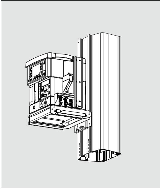
Fabius can be used in combination with the ceiling supply units Movita/Movita lift or Forta lift as a ceiling-mounted version. In this case, the anesthesia workstation is not placed on a trolley, (see chapter "Fabius Tiro as trolley version (front view)" on page 20), but rather on the mount of a ceiling supply unit.
