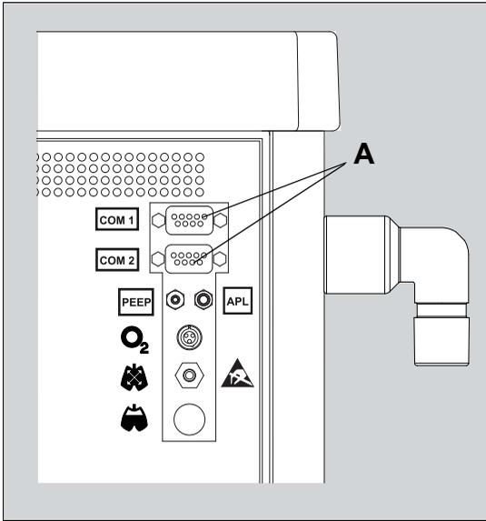
**A** There are 2 ports on the rear of Fabius for communication with external devices. The ports are marked with COM 1 and COM 2\*. These ports are used for data communication using the Dräger MEDIBUS or Vitalink data protocols.
