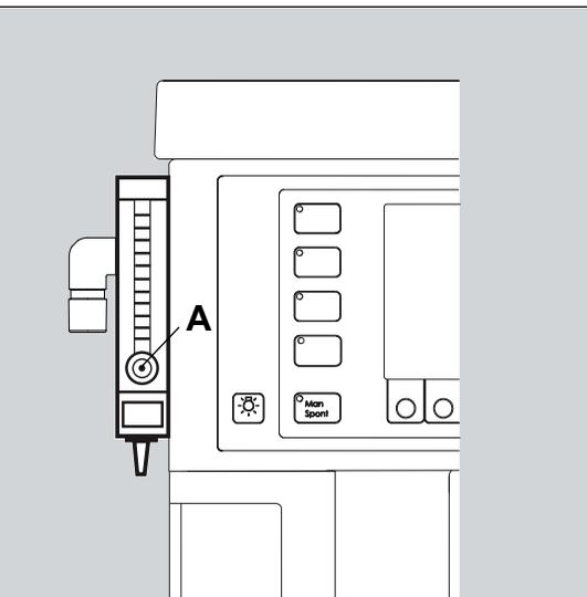
The supplemental O2 delivery supplies pure oxygen with an exact metered flow, e.g., for O2 insufflation using a face mask during a regional anesthesia. The supplemental O2 delivery is not only possible in standby mode and during operation, but also if Fabius is switched off.
