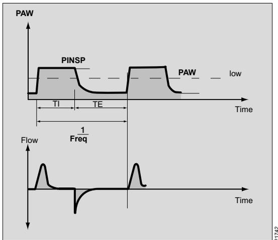
A tidal volume is supplied based on a defined respiratory rate (**Freq**) and a defined ratio of inspiratory time to expiratory time (**TI:TE**).
