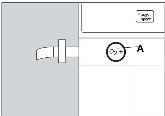
Use of the O<sub>2</sub> flush can increase airway pressure very quickly and abruptly change the gas concentration.
