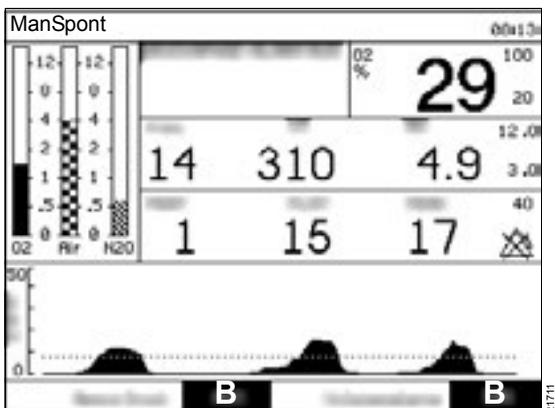
The following alarms can be activated or deactivated in **ManSpont** mode with the **ON/OFF** key (B):
