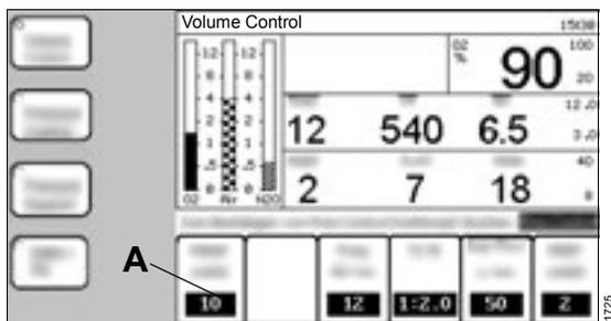
The ventilation settings for the new ventilation mode are automatically derived from the settings of the previous ventilation mode. The corresponding settings (A) in the new ventilation mode are highlighted.
