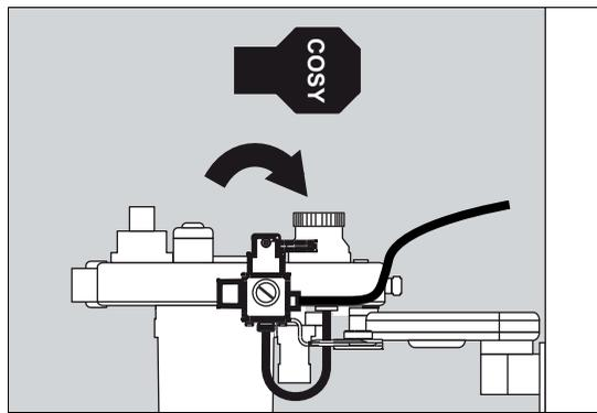
Diverting the fresh-gas flow to the compact breathing system:
