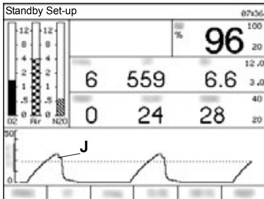
When the setting **Normal** is selected, the pressure waveform (J) is not shown as a filled area, but as a line.
