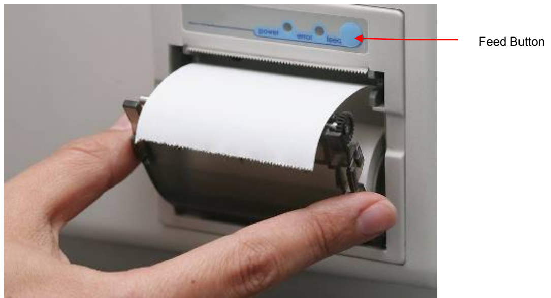
Figure 35 - Insert Paper Roll into printer
