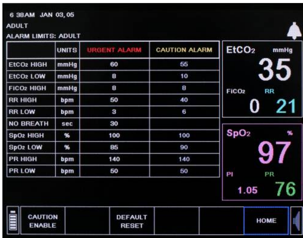
Figure 21 - Alarm Limits Screen
