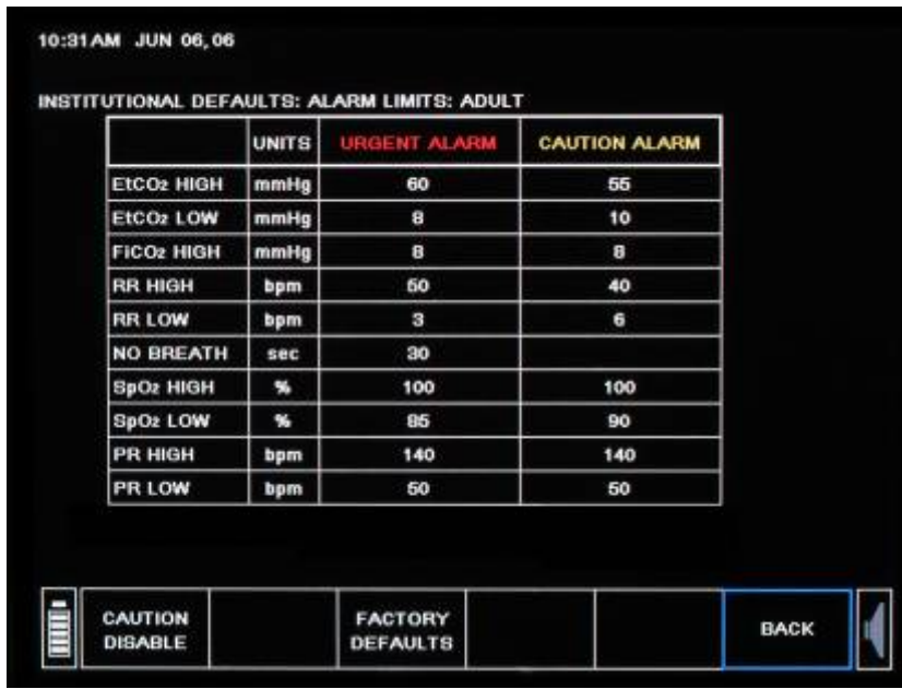
Figure 37 - Institutional Defaults Alarm Limits Screen
