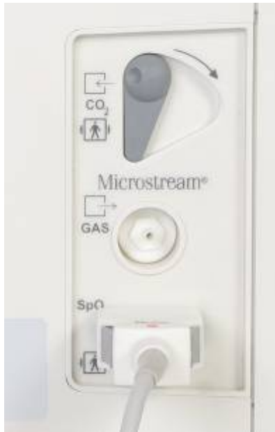
Figure 16 - Scavenger System Connection Point
