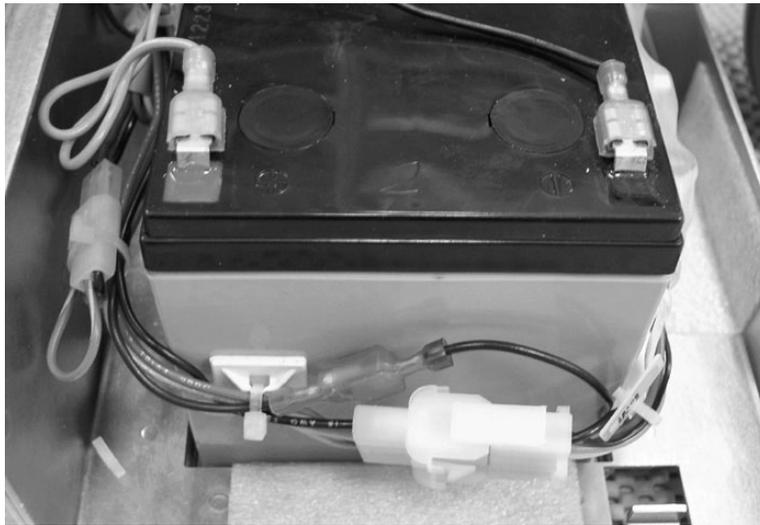
**Figure 3.8: Placing batteries into the tray**
