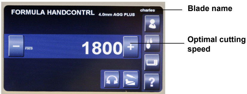
Figure 6A: The TPS Console screen after a 4.0mm Aggressive Plus blade has been inserted into the Formula Handpiece
