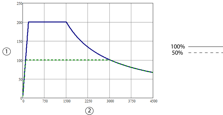
Output power versus resistance for BLEND power
