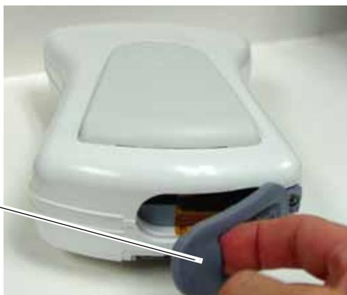
2. Pull the battery tray out of the Patient Data Module using the battery tray strap and remove the battery.
