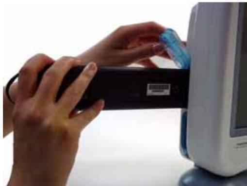
4. Gently push the battery door closed until it *snaps* into position. The battery door will not close if the battery is not fully inserted into the battery slot.
