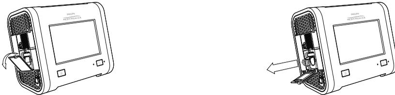
Verify the detachable battery is installed correctly. You should see the detachable battery icon appear in the Battery Power Meter on the Status Bar.
