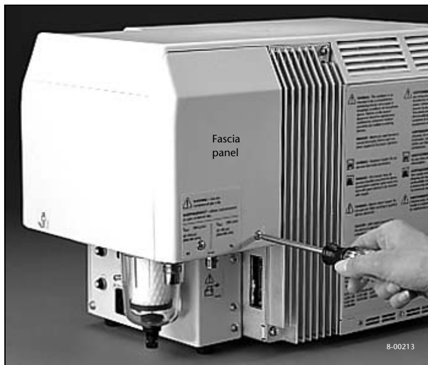
Figure 8-46. Removing inspiratory module fascia panel
