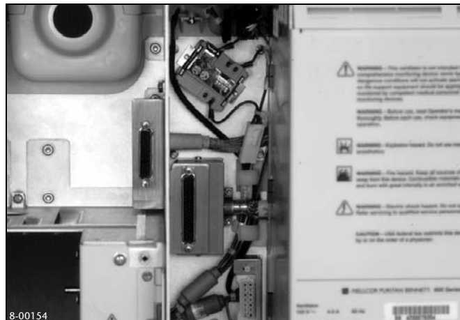
Figure 8-42. Replacing humidifier receptacle
