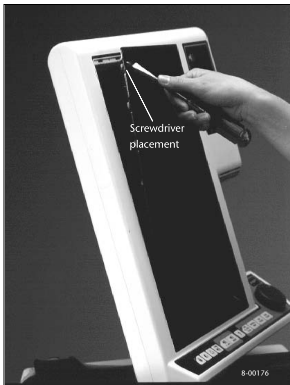
Figure 8-16. 9.4-inch touch screen bezel and window
