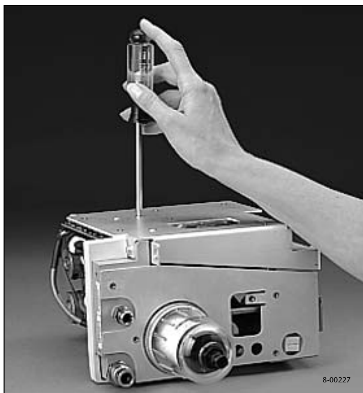
Figure 8-55. Removing inspiratory module right-side plate
