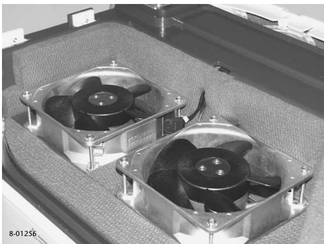
Figure 8-81. Fans installed in compressor
